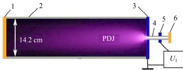
Fig. 1. Experimental setup diagram No. 1 with an inserted photo of the plasma diffusion jet (PDJ) glow obtained at an air pressure of 0.4 Torr and exposure of 0.25 s. 1 and 6 – capron flanges; 2 – tube made of ESALUX TX polycarbonate with an outer diameter of 15 cm and wall thickness of 4 mm; 3 – grounded electrode made of duraluminum with a hole for quartz tube 4 with an outer diameter of 21 mm and wall thickness 1.5 mm; 5 – external ring electrode made of steel foil with a width of 10 mm; U_1 – pulse generator with a voltage pulse amplitude at a load of U = +7 kV and frequency f = 21 kHz connected to electrodes 3 and 5
