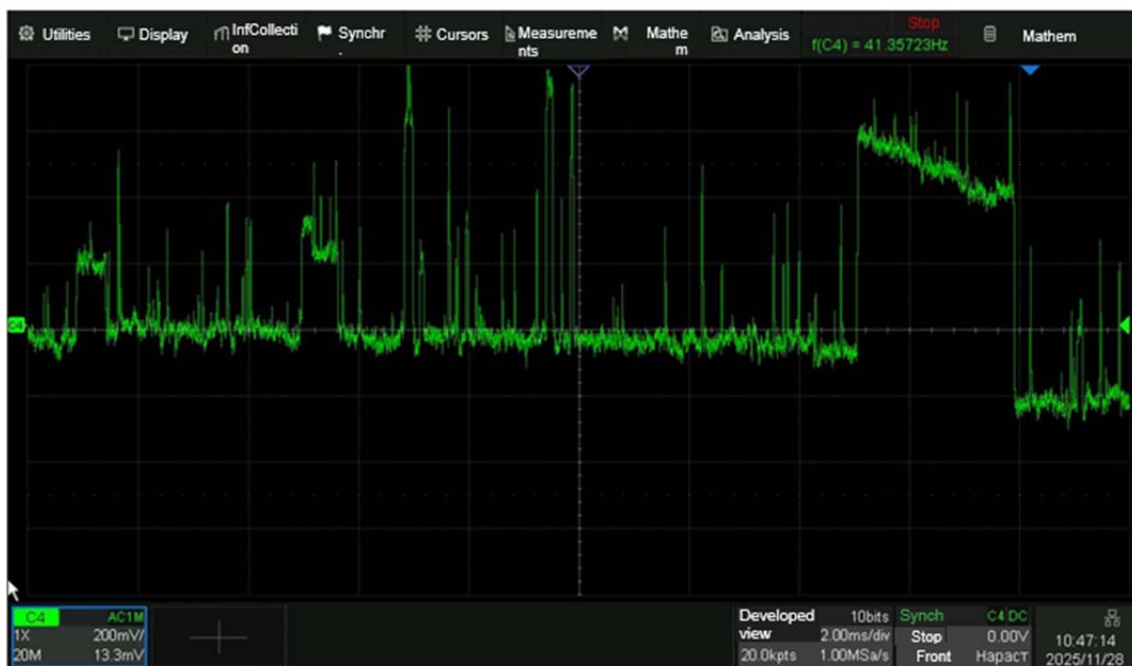
Fig. 4. Noise voltage oscillograms at voltages of 1 V and 10 V
