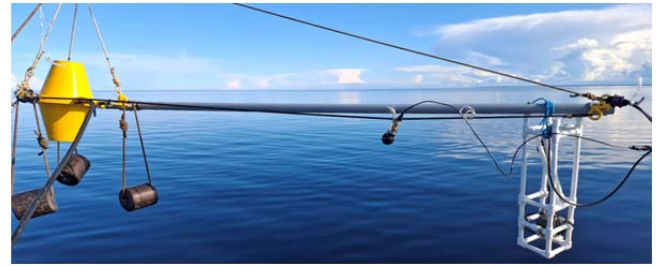
Fig. 2. Rig for measuring the electroacoustic characteristics of the 3D LF radiator
