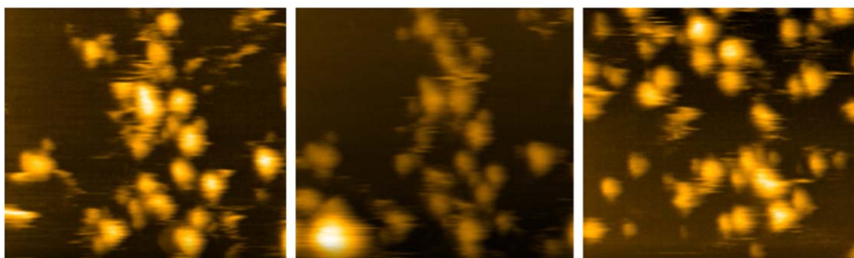
Fig. 2. AFM images of cytochrome P450 BM3 macromolecules in liquid, sequentially acquired with a high-speed AFM. Time per frame 1 s. Scan area 200 \times 200 nm. Height scale from 0 to 4.5 nm. Frames were acquired at time points 0 s (left), 23 s (center), and 60 s (right)
