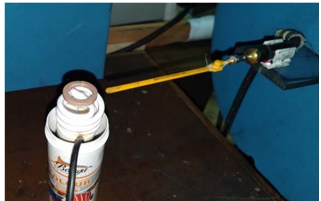
Fig. 1. Photo of the dielectric ring system on the spiral lamp. The magnetic field probe is located on the right
