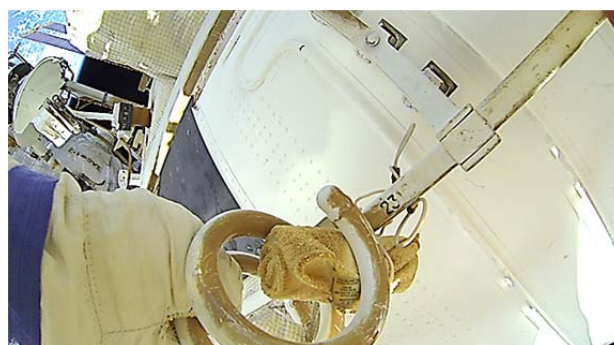
Fig. 3. A cotton fabric bundle secured on the painted external surface of the Service Module of the ISS RS
