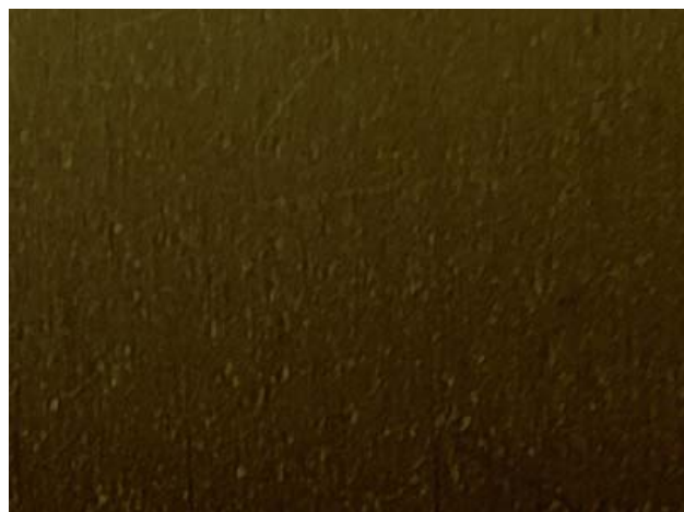
Fig. 3. Surface of the sample with the deposited 2DO LCC + Li layer after testing. No fungal growth is observed. Magnification – \times 10
