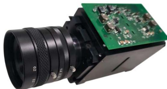
Fig. 8. Appearance of the photodetector optoelectronic television channel of the active-pulse OUVS based on the FPM-5-1 type module
