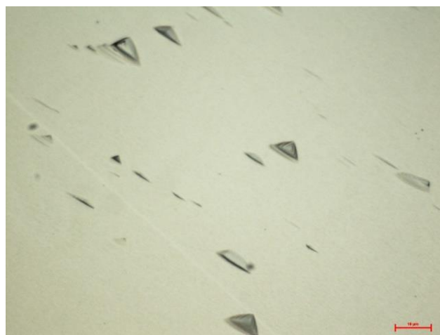
Fig. 10. Typical view of the dislocation pattern of the single-crystalline region of a CdZnTe wafer (211)B after selective etching
