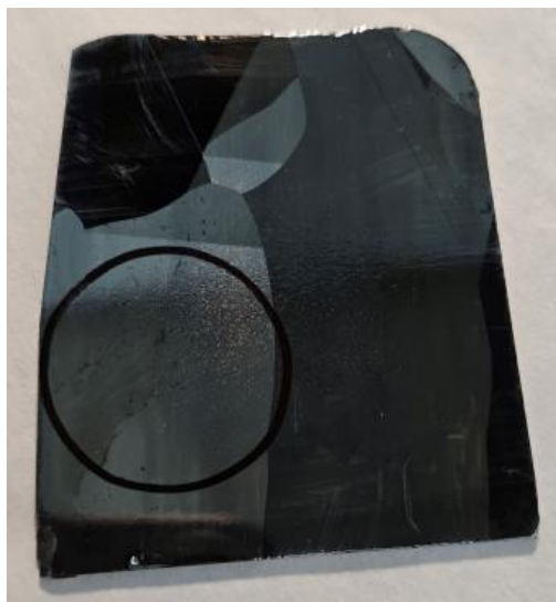
Fig. 9. Appearance of a CdZnTe wafer (211)B after selective etching. The contour marks the single-crystalline region on side B of the cut wafer section
